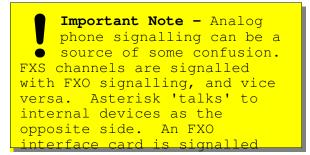
with FXS signalling by Asterisk, and should be configured as such.
