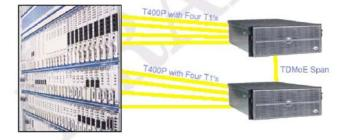
Asterisk can be used as a high density IVR and conferencing platform, using traditional PRI/T1 interfaces, and providing redundancy, scalability, and intercommunication using TDM over Ethernet, which permits Asterisk to extend the TDM bus across the ethernet network, while retaining minimal latency.
