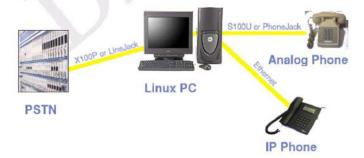
One question that is often heard is "How small of a PBX can you build with Asterisk?". Well, you can make a PBX as small as one port of PSTN and one port of analog or IP phone. Yes, it is true that you can make a PBX with just one port, but it isn't very useful unless
