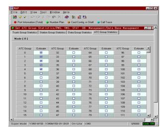
Select the ATC to collect Statistics and press the [Tx] button.
