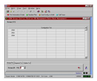
2. Configurate the ISDN Group to collect Statistics and press the [Tx] button. One ISDN Group can configurate 16 Groups.
