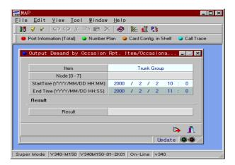
3. Press the [Tx] button to save data. Then the phrase 'Print Request Completed' will appear in the 'Result' window and the report will be printed by the printer connected to the system.
