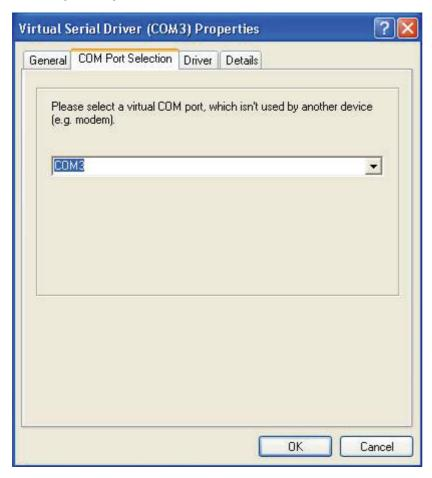
Select a virtual COM port (COM1-COM16) for the telephone which is not being used for another device (such as a modem). Click **OK**.
