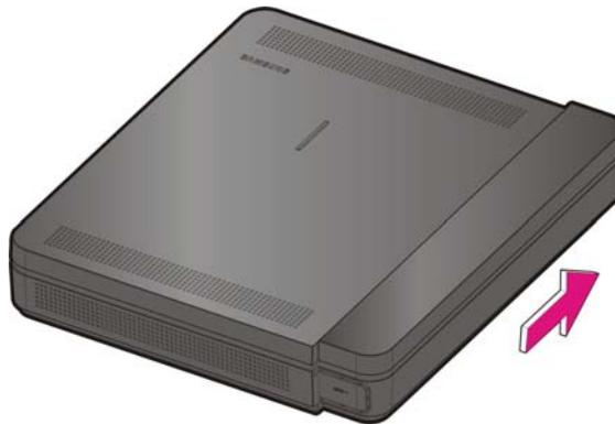
Figure 2.1 Removing the cable duct cover (1)
