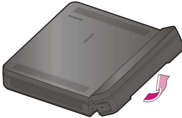
**Figure 2.2 Removing the cable duct cover (2)**
