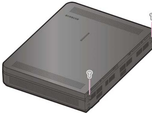
Figure 2.17 Installing the top cover (2)
