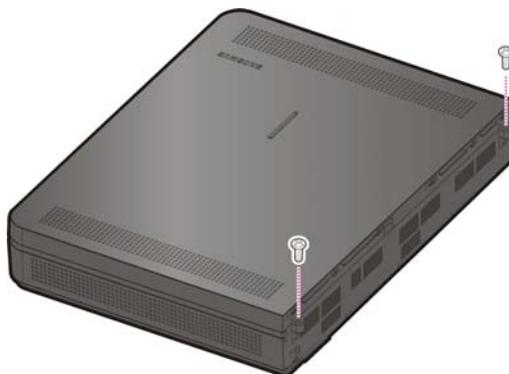
**Figure 2.4 Removing the screws**
