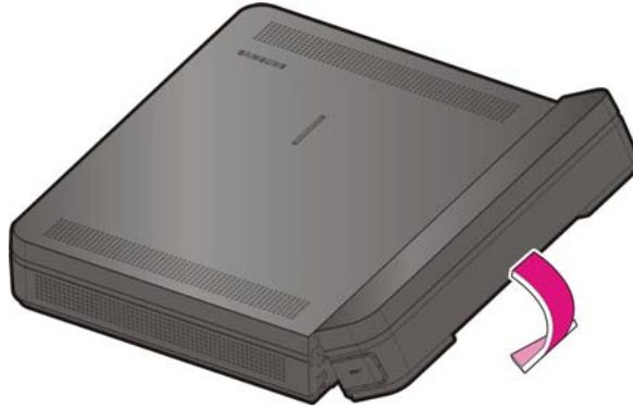
**Figure 2.19** Installing the duct cover (1)
